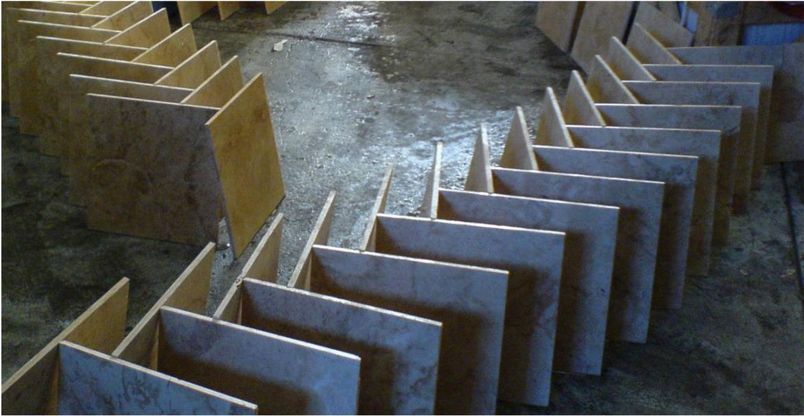
In the picture above we can see that this method will allow air to the tiles so that they can dry.
